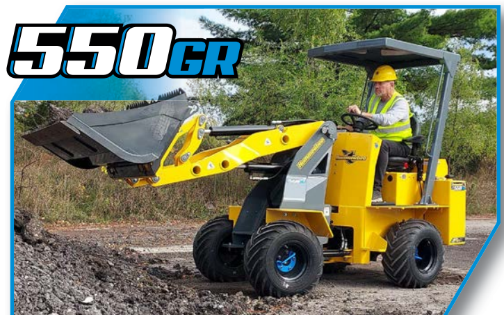
Same Features as the 525R, Plus: 50 HP Kubota WG1605 Liquid-cooled Gasoline Engine; Same Durability as a Diesel Engine, but Quieter; 88.51 ft-lbs of Torque; 29x12.50x15 Tires.
